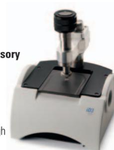
The **iD3 ATR accessory** provides exceptional single-bounce ATR performance at an attractive price. The iD3 features very high sensitivity with its high-throughput 7 mm crystals (ZnSe or Ge), while maintaining exceptional line shapes of absorbance bands.
